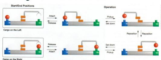
Just like a macroscale assembly line robot the nanotransporter can pick up, move and release a small molecule cargo
